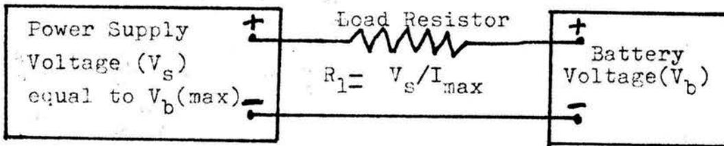
A) Constant Voltage Charging System, requires power supply closely matched to battery voltage. Its advantage is that you don't have to keep track of charging time.
