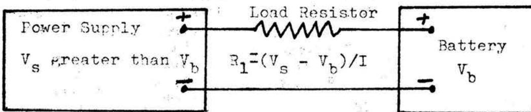
B) Constant current charging system, Cheap, will work with a variety of different batteries, or numbers of cells. You must keep track of charging time to prevent overcharging.
